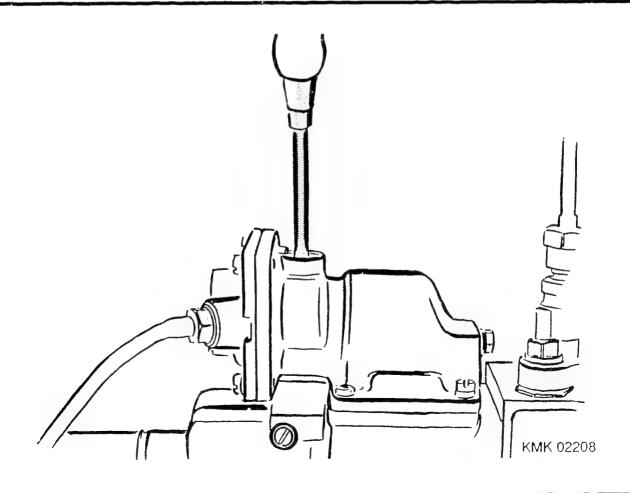
\* Checking LDA characteristic-curve profile.
